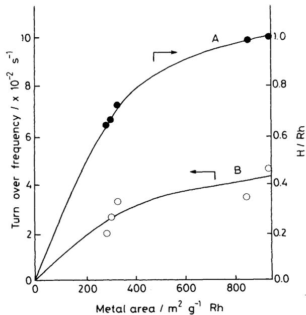
**Figure 3.** A correlation between metal area, dispersion (●), and turnover frequency (○) for aniline hydrogenation.
